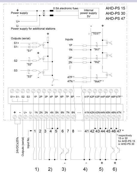
Example 1) Acquisition of 2 binary contacts with 2-pole connection.
