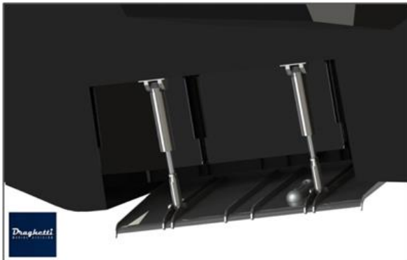
Customized trim tab with two cylinders
